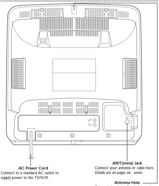
Connect the stem of an indoor antenna here. *Details are on page six.*
